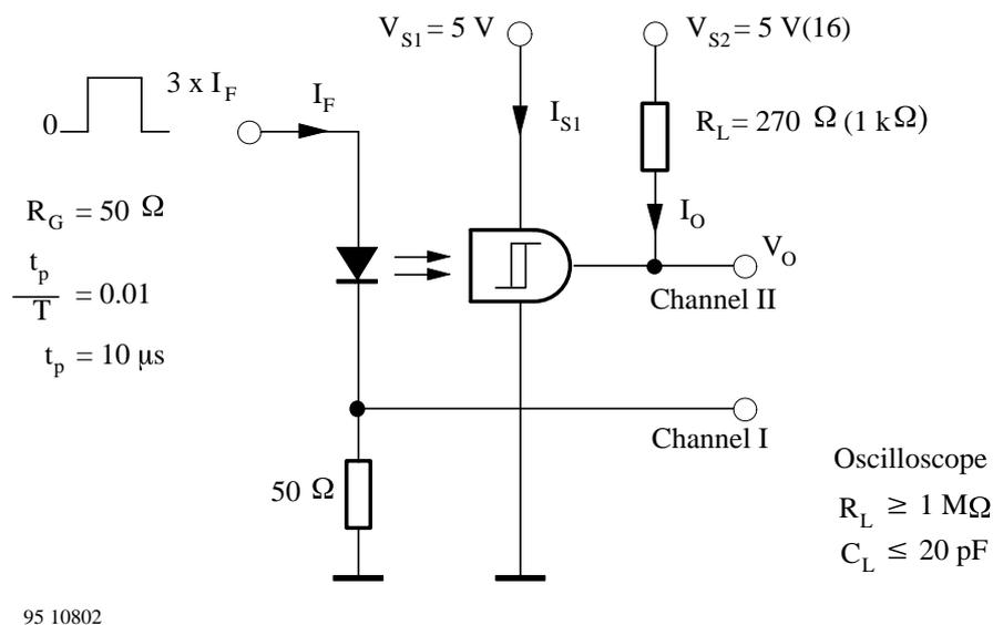
Figure 1. Test circuit
