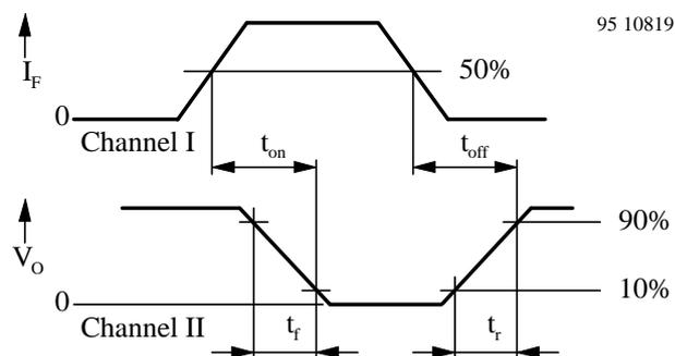
Figure 2. Pulse diagram
