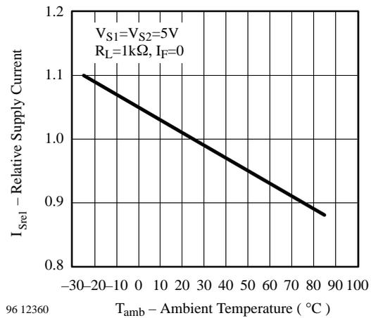
Figure 6.  $I_{srel}(T_{amb})$
