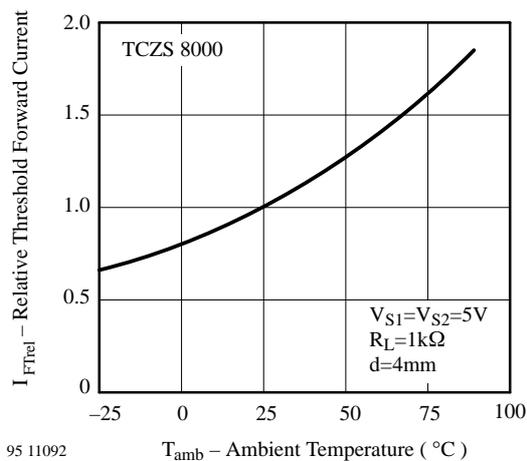
Figure 5. Rel. Thresh. Forw. Current vs. Ambient Temperature
