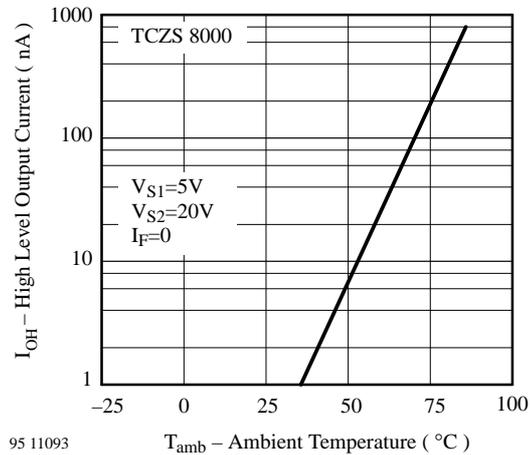
Figure 7. High Level Output Current vs. Ambient Temp.
